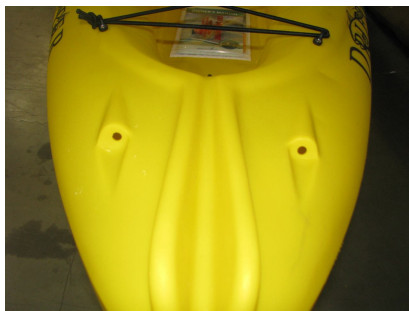
Fig.#C Stern Cable Holes
